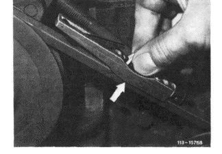
3 Exert a uniform, vertical pressure on V-belt upper surface by means of pushbutton, until click spring is audibly (or noticeably) disengaging.
