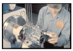
41. When you measure rack position, you are setting the position of each plunger helix in its barrel.
