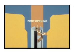
37. Right, by changing port opening, when the plunger helix uncovers the port. At port opening, pressure falls to supply pressure, shown in orange. With no delivery pressure, injection stops at the cylinder.
