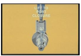
25. When we rotate the cam to a specified lift to port closure, we establish a zero check point for pump timing.
