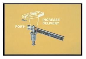
47. Let's see if we can put it all together. In calibration, to increase delivery, turn the barrel and port this way in relation to the plunger helix. In operation, the rack turns the plunger the other way in relation to the port.
