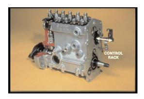
14. ... each one manages the M-W pump by moving the control rack to meter delivery to the injectors. We all know that, when the rack moves . . .
