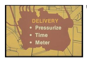
53. In this program, you've seen that pump delivery involves three jobs: to pressurize the fuel, to time the injections, and to meter the quantities delivered.
