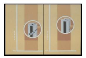
38. On the left, you can see that, when the helix uncovers the port sooner in the stroke, less fuel is delivered. In comparison, when the helix uncovers the port later in the stroke, more fuel is delivered.
